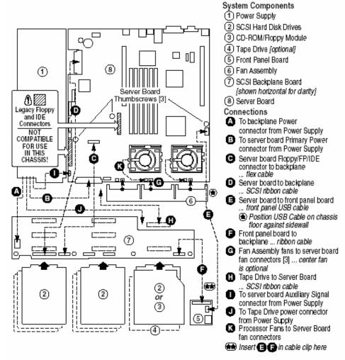
Figure 12: Routing Cables
